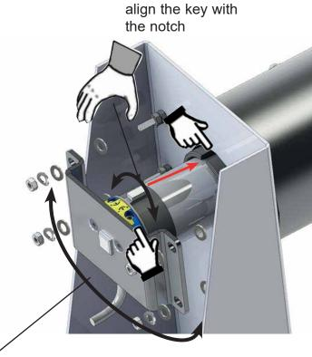
Make small rotating movement with the motor to facilitate the insertion
