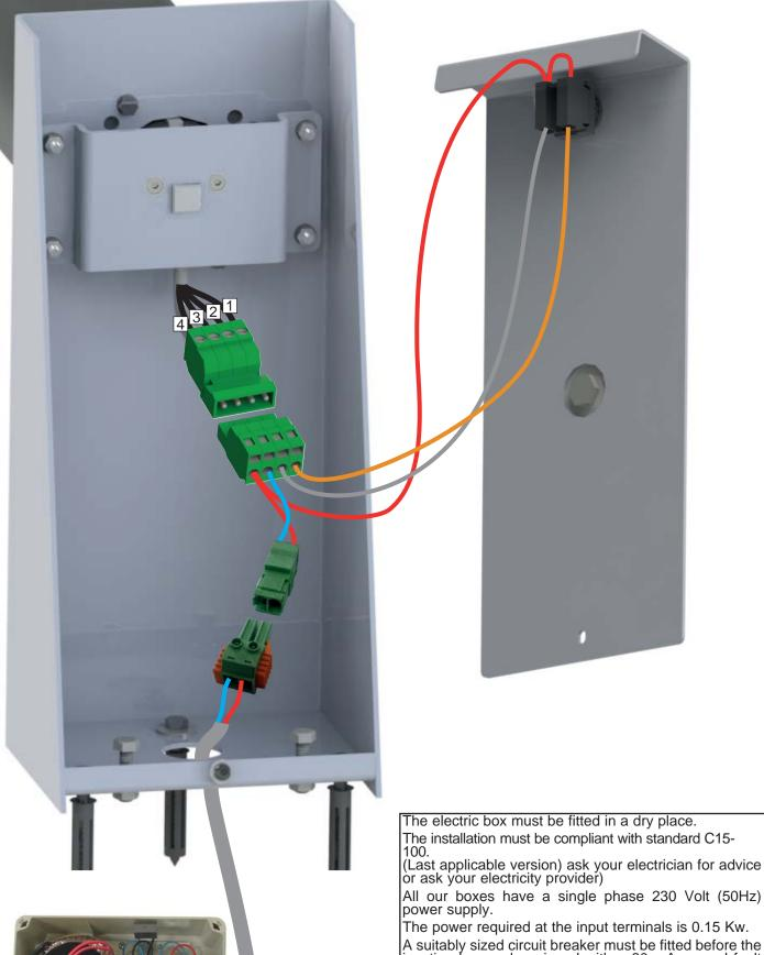
A suitably sized circuit breaker must be fitted before the junction box and equipped with a 30 mA ground fault
