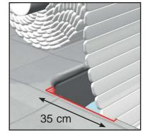
If necessary, cut the sides to ease the passage of the cover and avoid rubbing
