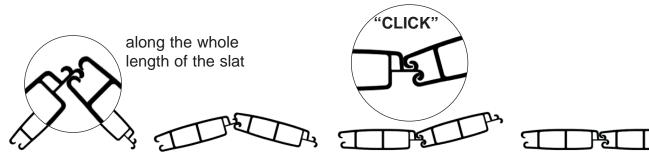
Repeat the movement until all the slats are completely clipped together
