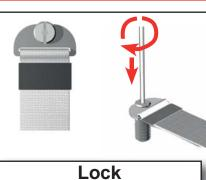
Lock the eyebolt The strap must be tight and the cover must touch the bottom of the straplock
