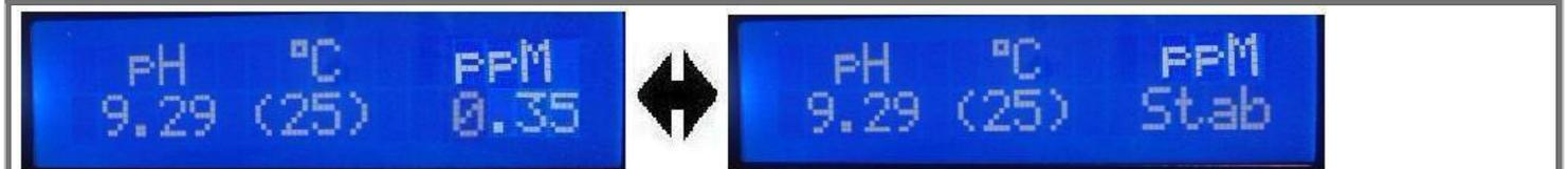
**WHAT IS IT?** It's a control that DUAL performs when it is switched on that allows the system to stabilize the pH before dosing the chlorine or activating the CL power plug on DUAL pH/CL REG.
