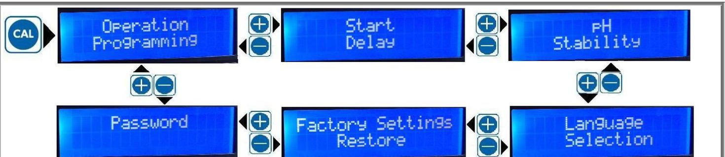
Push and quickly release **CAL** button during the functioning to enter into the programming menu. Push + or - button to navigate through the menu. Push the **CAL** button to enter the submenus.
