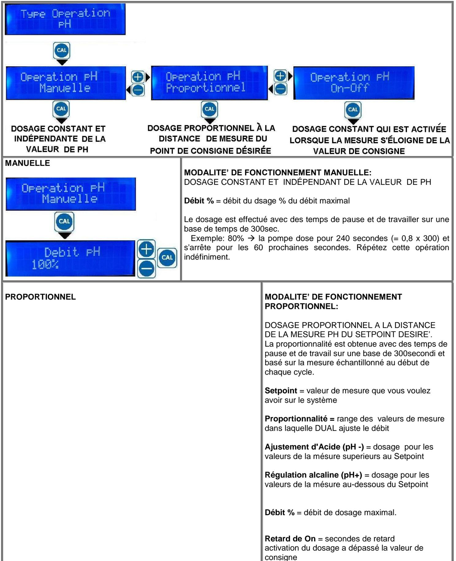
The screenshot shows a vertical menu of settings for a pH proportional control system. Each setting is displayed in a blue box with white text. Navigation is done using a 'CAL' button (down arrow) and '+'/'-' buttons (right side of the boxes). The settings are:
