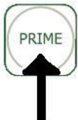
**UK** Keep pressed PRIME button to prime the pump. The red level led lights up and the display scrolls the reading StArt. When the button is released the pump goes back in the state congruent with the actual inputs.
