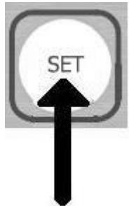
**UK** To read the values of the setpoint data (setpoint, ACD / bAS) push shortly the SET button. The SET led will start blinking and the display will show for 3 seconds the value of the previously stored setpoint, then the display will show for 3 seconds the stored Acd or bAS values. The SET led will turn off and the display will go back to measurement.
