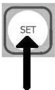
**UK** To read the values of the memorized data (CAP,FH) push shortly the SET button. The 3 led will start blinking and the display will show for 3 seconds the value of the previously stored CAP, then the display will show for 3 seconds the stored FH value. The 3 led will turn off and the display will go back to actual functioning.
